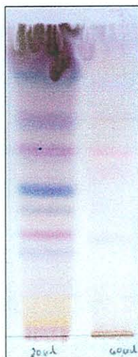
Figure 3.1 Chromatogram showing the separation of compounds present in 380 µg of the acetone extract (left) and 408 µg of the bicarbonate extract (right). The CEF system was used as eluent and the plate was sprayed directly after TLC with the vanillin spray reagent.
