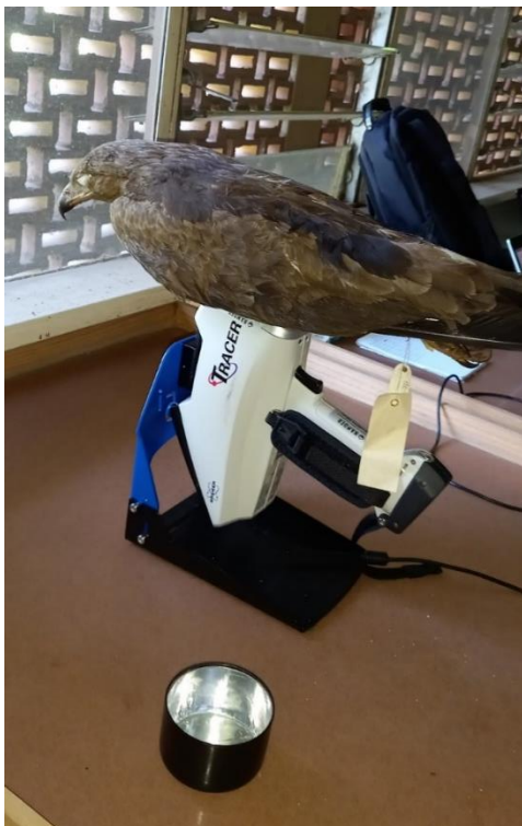
Figure 2. Positioning a taxidermy specimen on the spectrometer. Natural History Museum of Zimbabwe. Photo: Maggi Loubser
