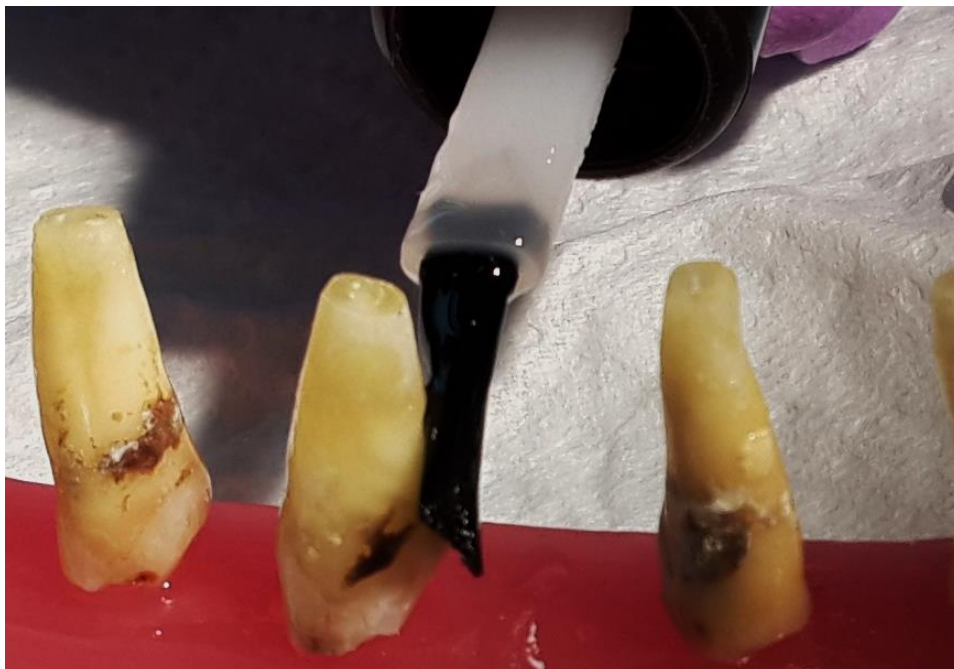
Figure 3.17: All the specimens were coated with two layers of clear nail varnish, except for the resected apical end.
