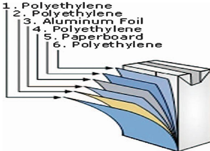
Figure 4 Schematic diagram of the individual layers making up the multilayered Tetra Brick ® (Tetra Pak, 2008). (color figure available online.)
