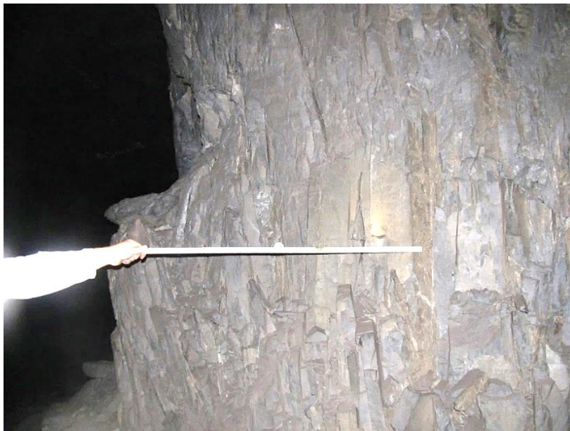
Figure 11-4. Joint spacing on the left-hand corner of Side A. The spacing ranged from 5 cm to 20 cm.
