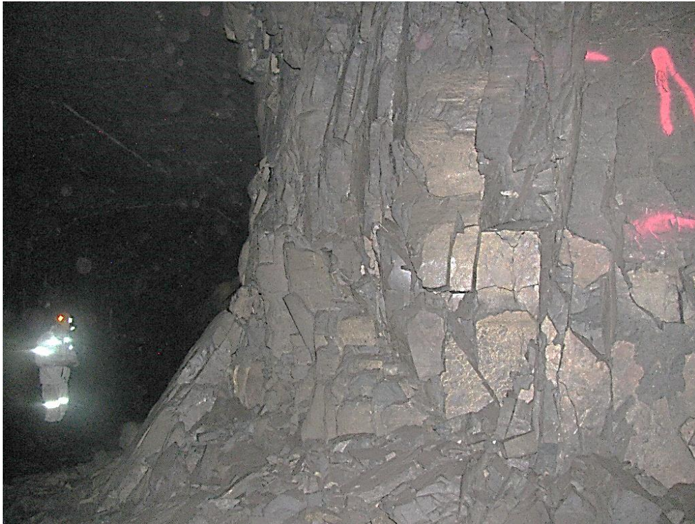
Figure 12-13. Side A of pillar N3_2 at Nchwane III shaft illustrating the vertical joint sets on the left-hand corner of the pillar.
