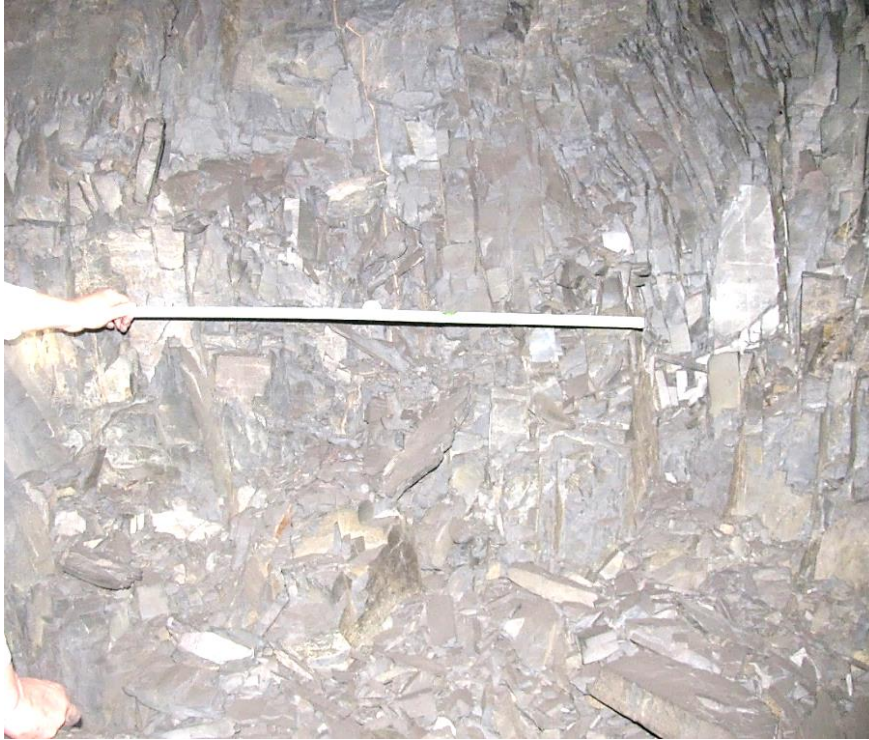
Figure 11-5. The vertical joint spacing on the right-hand side of the pillar. It was difficult to determine as the spacing of the joints as it varies across the perimeter of the pillar.
