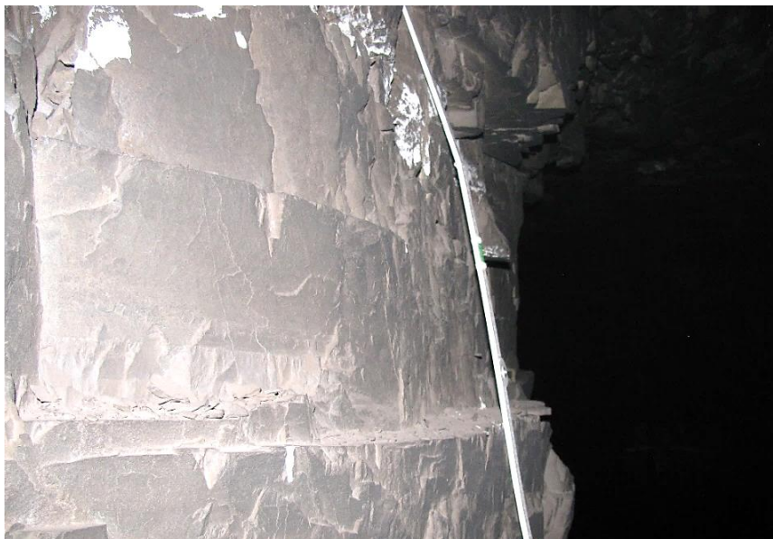
Figure 3-17. The horizontal joint spacing of side C ranges from 15 cm to 25 cm.
