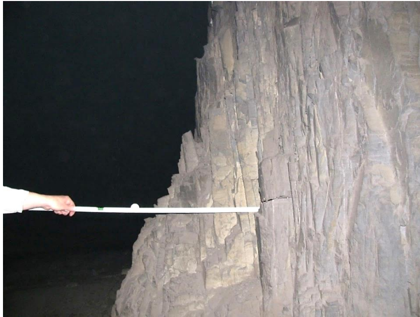
Figure 3-16. The pillar corner at side A illustrates the vertical joints with a spacing of 1 cm to approximately 6 cm.
