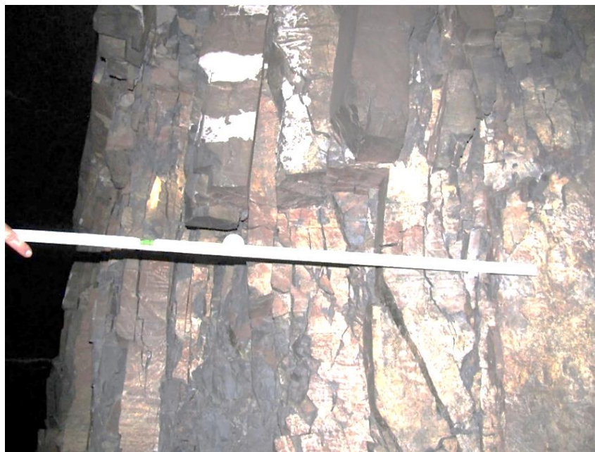
Figure 3-19. Side A of pillar N3_25 illustrates the joint spacing in the vertical direction.
