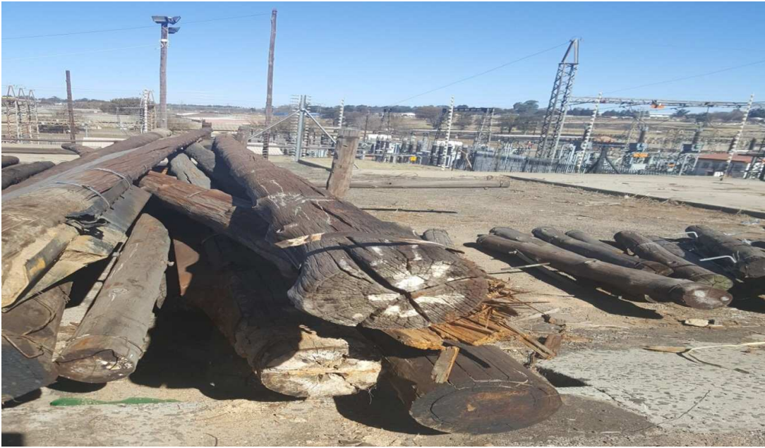
Figure 4.5: Rotten wooden poles, Ermelo CNC – Ermelo Zone
