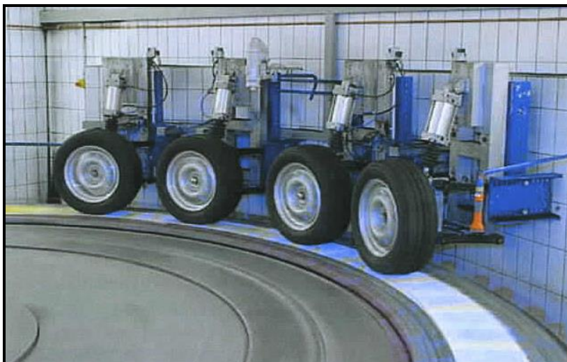
Figure 2.4: Turntable road marking test system (Zedler, 2014).
