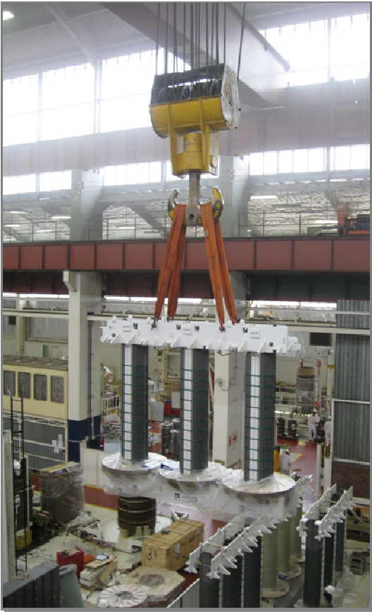
Figure 1.3: Cores are transported via the overhead crane
