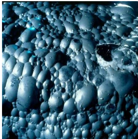
Figure 21: An illustration of the froth at the surface of the pulp in a flotation cell (metallurgy.utah.edu, 2008)
