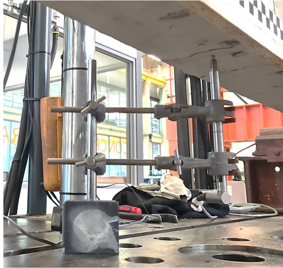
Figure 3-4: LVDT installed beneath the beam for mid-span displacement measurement
