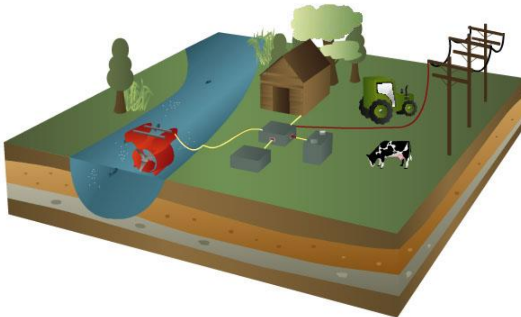
Figure 1-2: Basic concept of HK systems (SHP, 2016)
