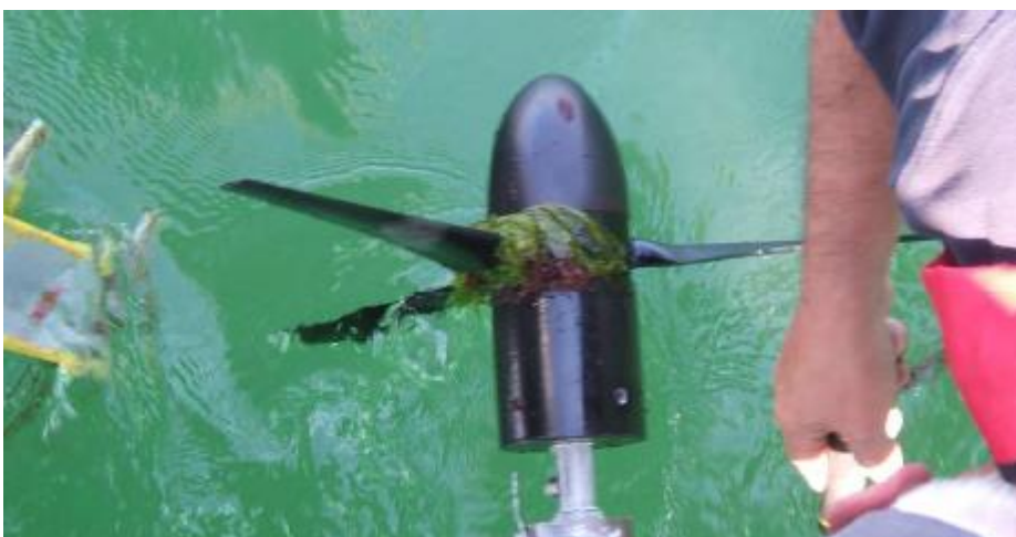
Figure 2-30: Weeds on turbine in the UK (Anyi, 2013)
