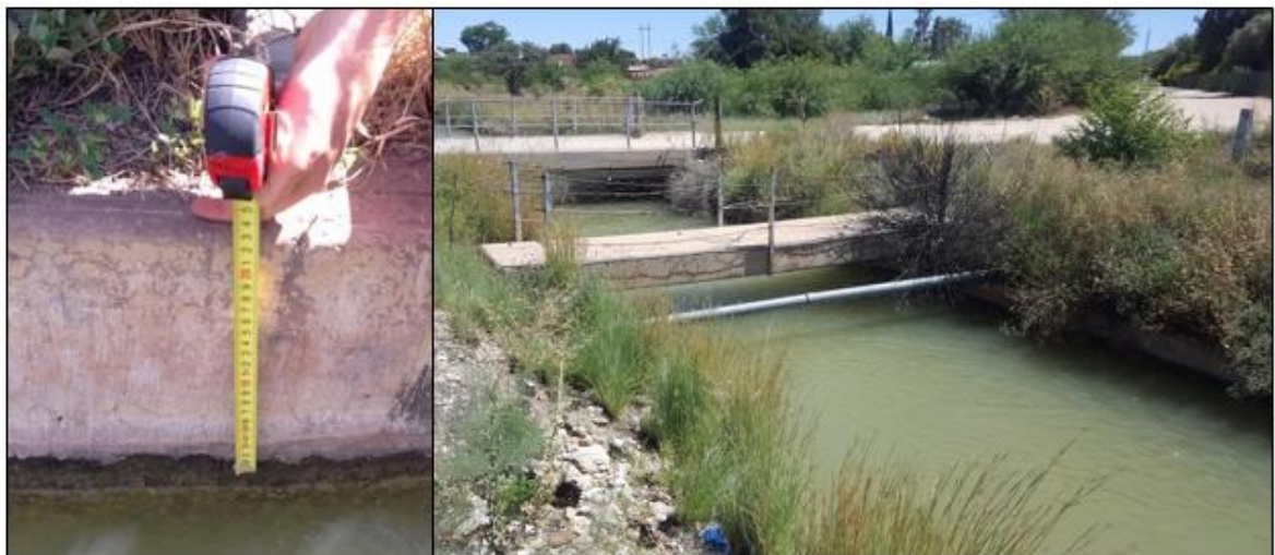
Figure 3-13: Water depth measurements at sites
