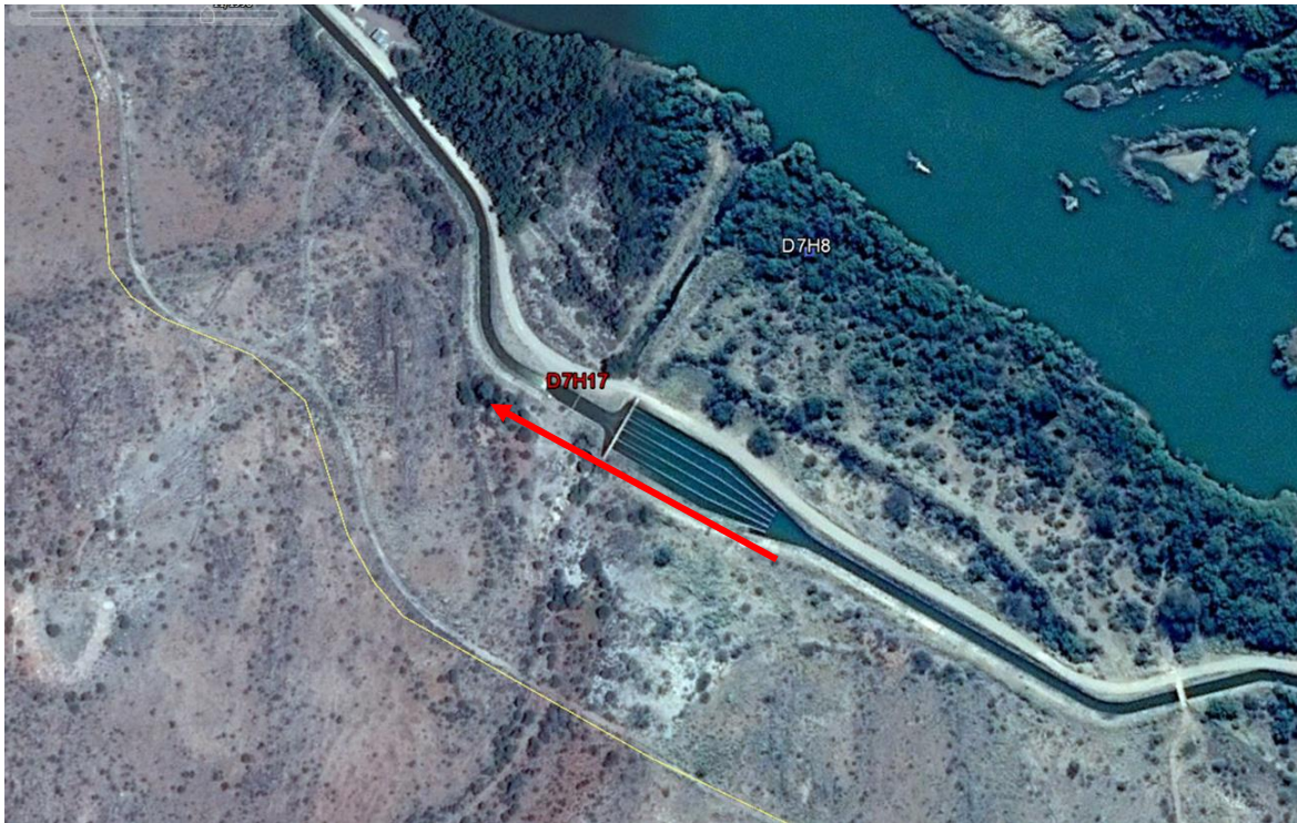
Figure 3-5: Gauging station D7H17 on the Boegoeberg canal system (flow direction indicated) (Google Earth, 2016)
