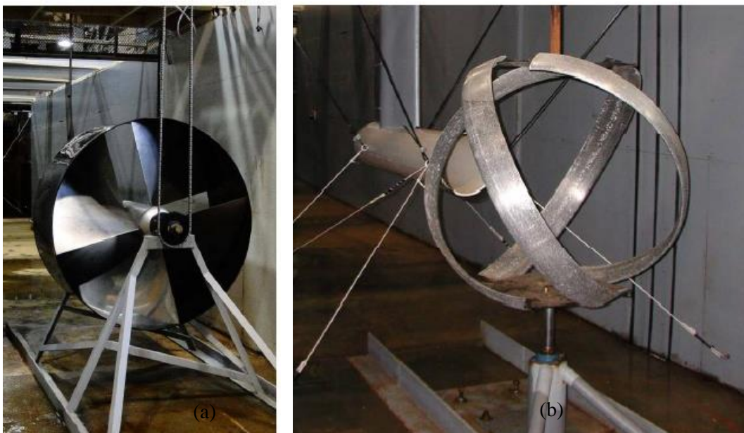
Figure 2-31: Turbine proving as “fish-friendly” (a) Welka UPG turbine (b) Lucid spherical turbine (Jacobson, et al., 2012)
