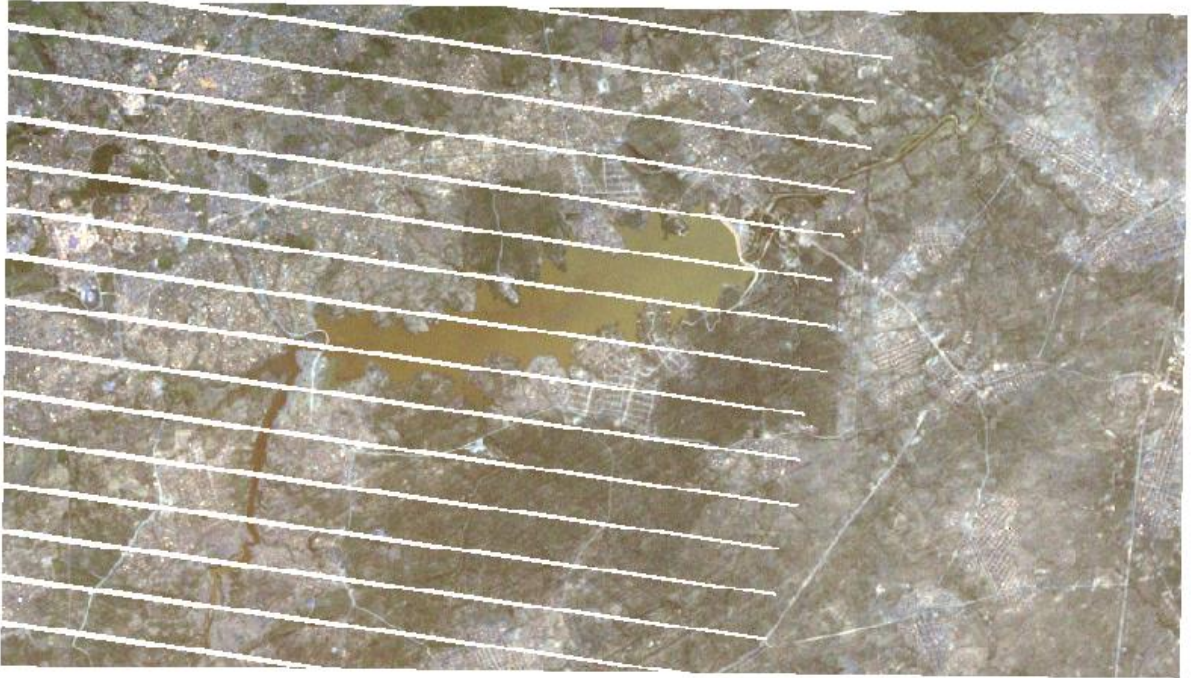
Figure 12: SAR, Current slicing Sensor Issue in Landsat 7 Sensors.
