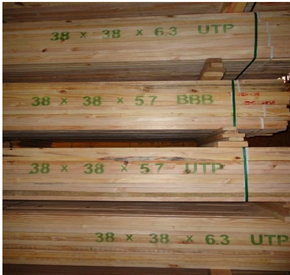
Figure 1: Different grades stacked together.
