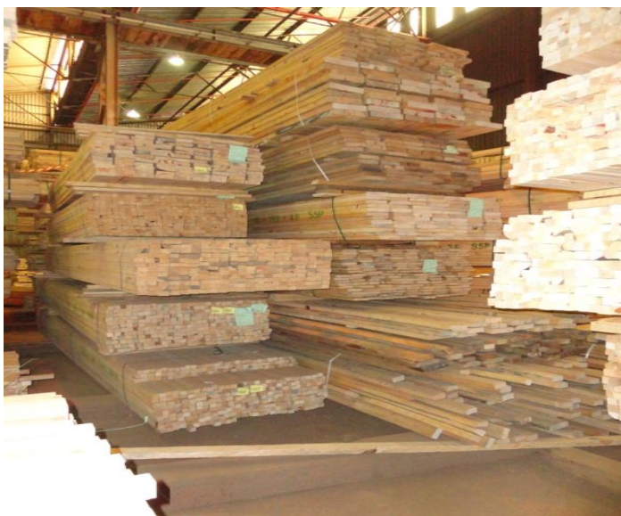
Figure 5: Safety hazard: products are not properly stacked.
