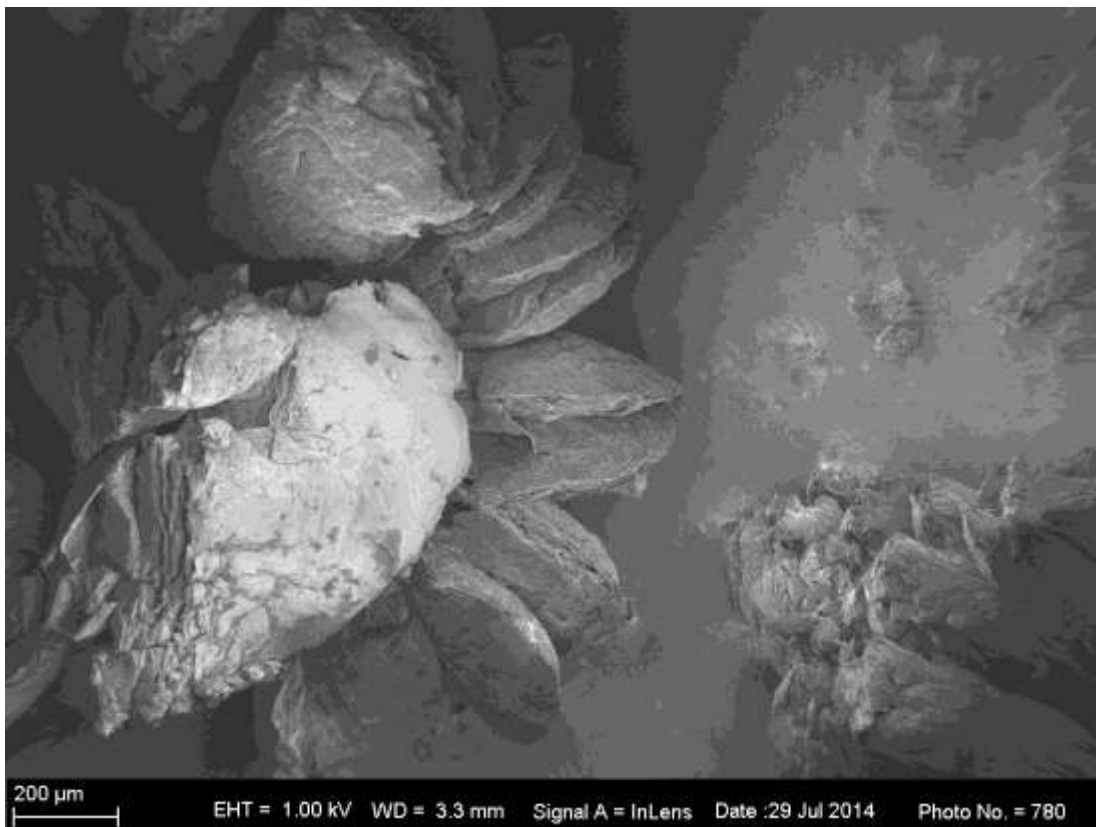
Figure 4-42: SEM of the worst gas expanded sample (140x magnification).
