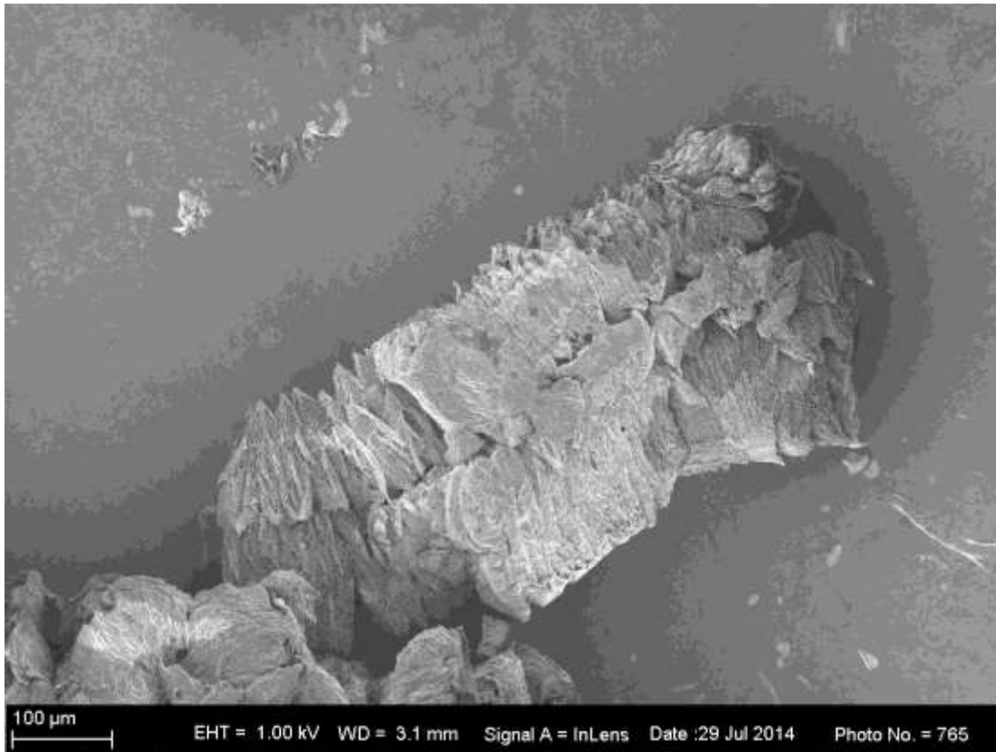
Figure 4-35: SEM of the electrochemical expanded sample (300x magnification).
