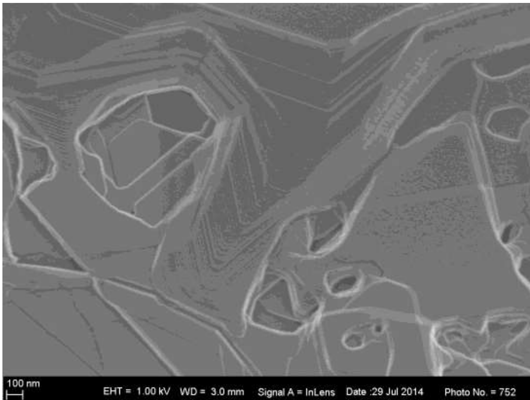
Figure 4-81: SEM of purified best gas phase sample (90000x magnification).
