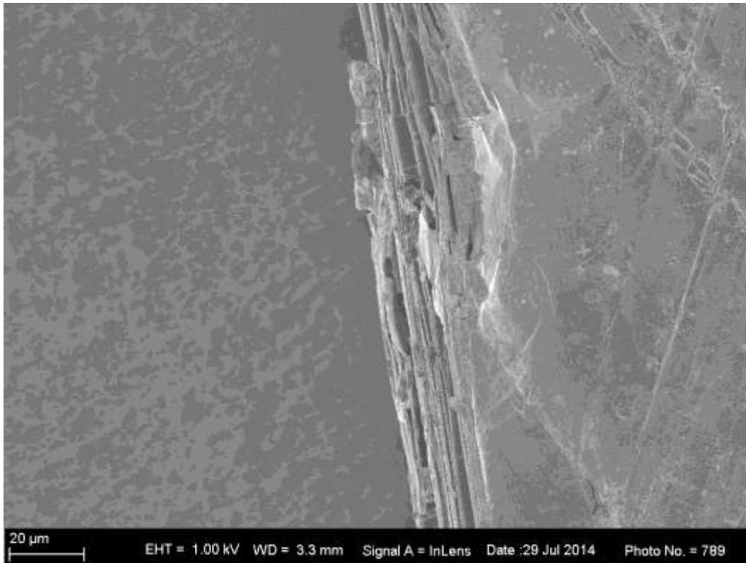
Figure 4-14: SEM image of electrochemical intercalated sample (1500x magnification).
