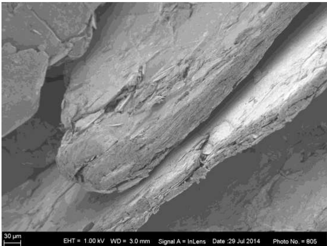
Figure 4-23: SEM of the worst gas phase intercalated sample (500x magnification).
