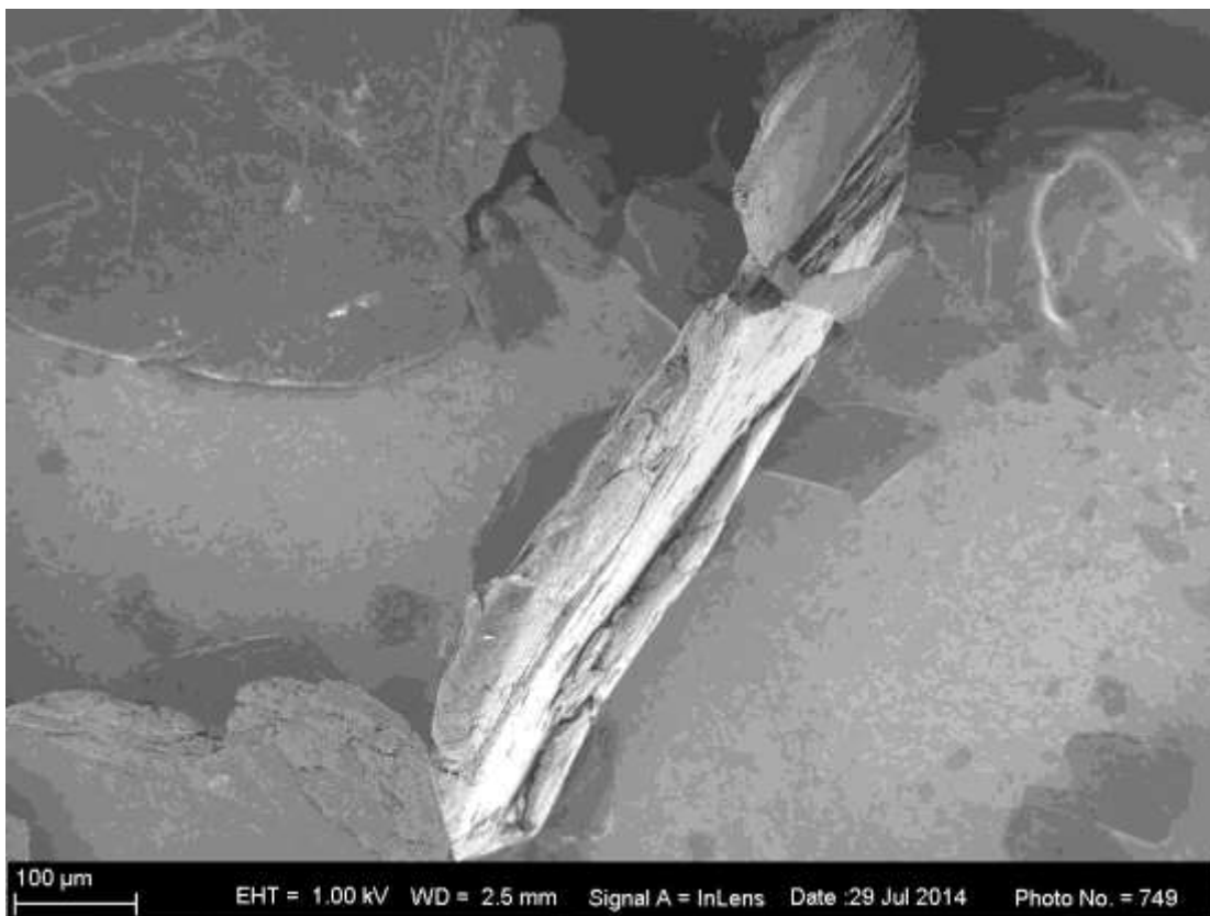
Figure 4-10: SEM image of the graphite flakes as received (300x magnification).
