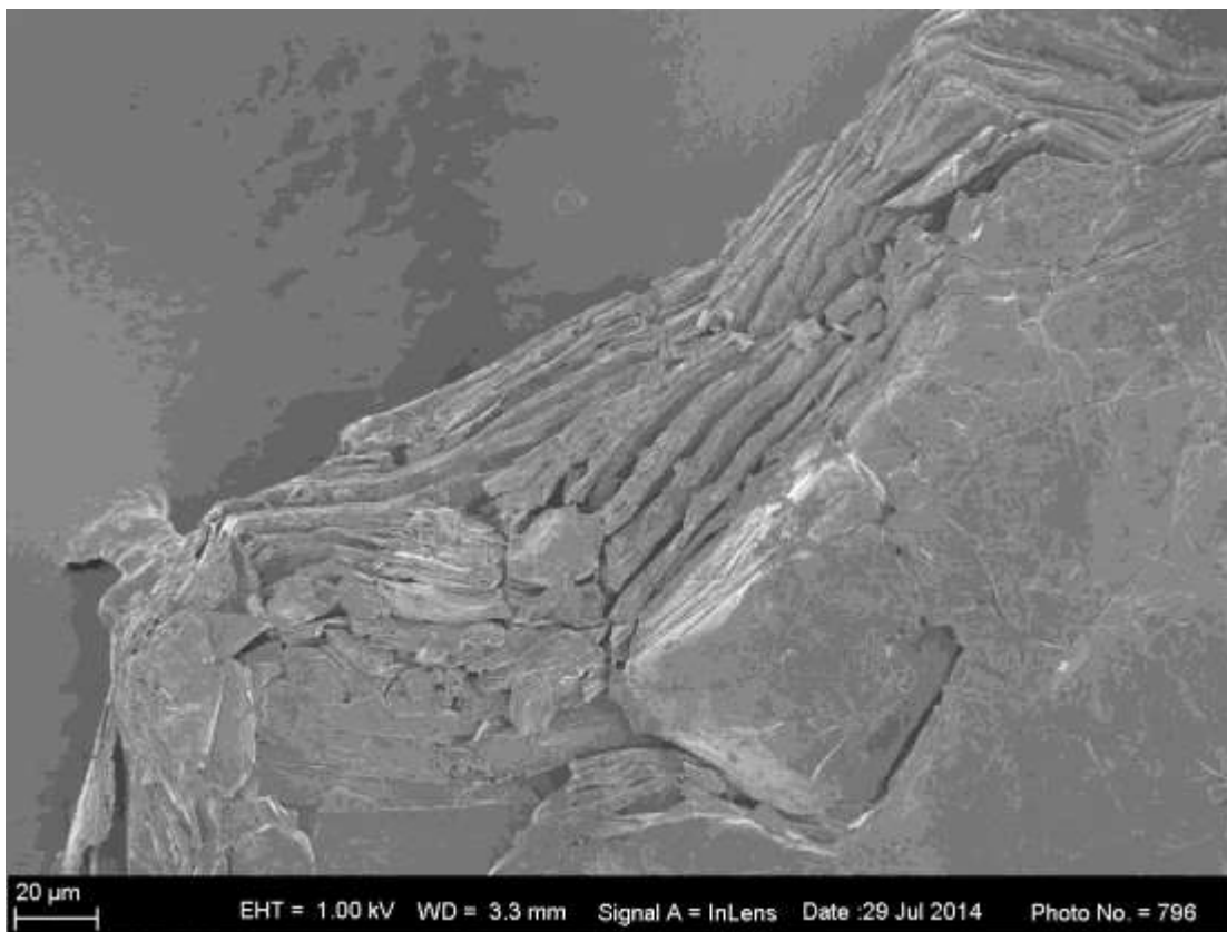
Figure 4-33: SEM of the worst Hummers intercalated sample (1000x magnification).
