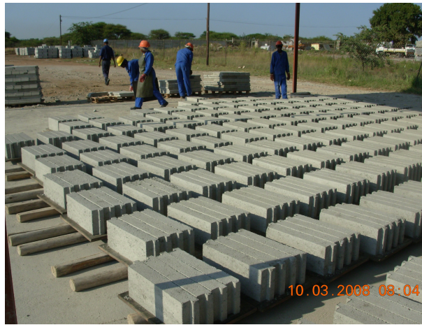
Figure 24 - FT 90 Block Production
