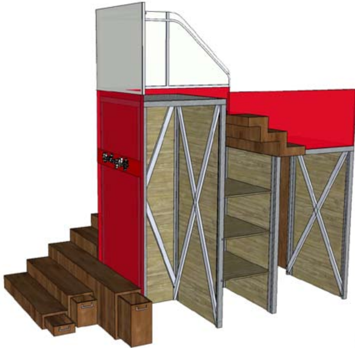
Figure 89(b): Back of staircase, showing storage facilities
