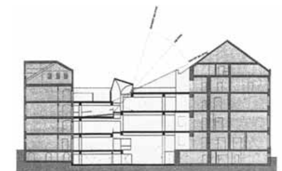
Figure 5.30. The resolution between the varying levels of the two historic buildings. (Holl, 2010)
