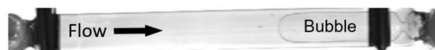
Figure 12: Snapshot of a high-speed flow visualisation video during flow boiling in a microchannel.
