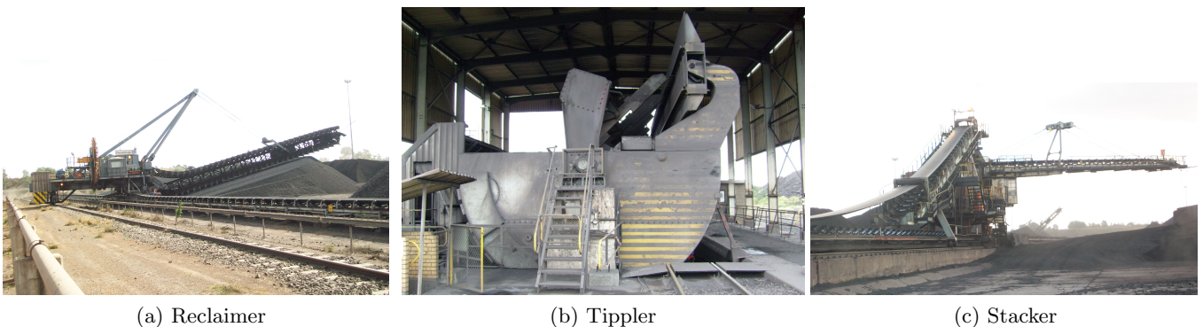
Figure 3.1: Main components of the RMTS
