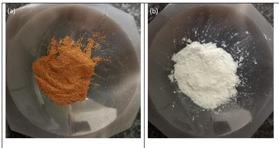
Figure 9.4: The precipitation products from the leachate of the 450°C roast, after filtration at (a) pH of 7.0 (product E) and (b) pH of 11.0 (product B).
