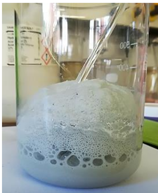
Figure 6.1: Impure talc reacting with 10% HCl solution to remove carbonate minerals.
