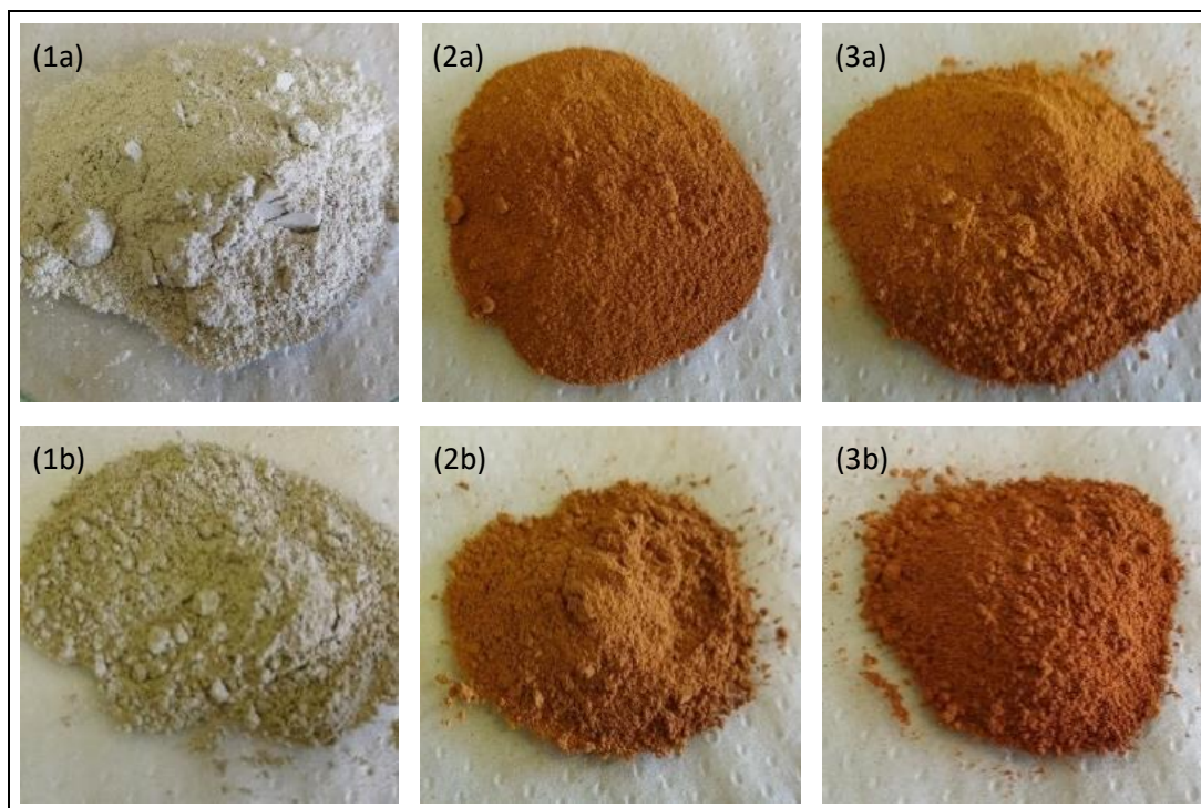
Figure 8.10: Comparison of (a) the colour of roast products for temperatures (1) 450°C with AS, (2) 450°C with AS + 680°C and (3) 450°C with AS + 750°C, and (b) the corresponding leach residues for (1) 450°C with AS, (2) 450°C with AS + 680°C and (3) 450°C with AS + 750°C.
