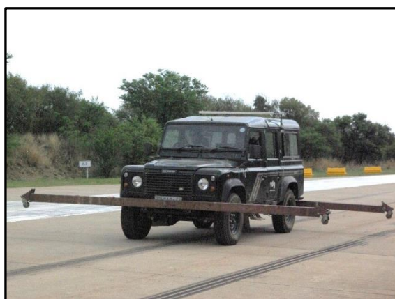
Figure 3-13: The Land Rover Defender 110 on the Belgian paving at Gerotek (Poovendran, 2018)
