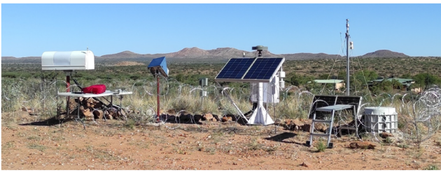
FIG. 23. Remote sensing instruments installed at H.E.S.S. From left to right panels: WVR-III+, Survey 3, solar panel, and GNSS station. Note that the radiometers are pointed toward the south because of the unobstructed view to the horizon, which favors the measurements.
