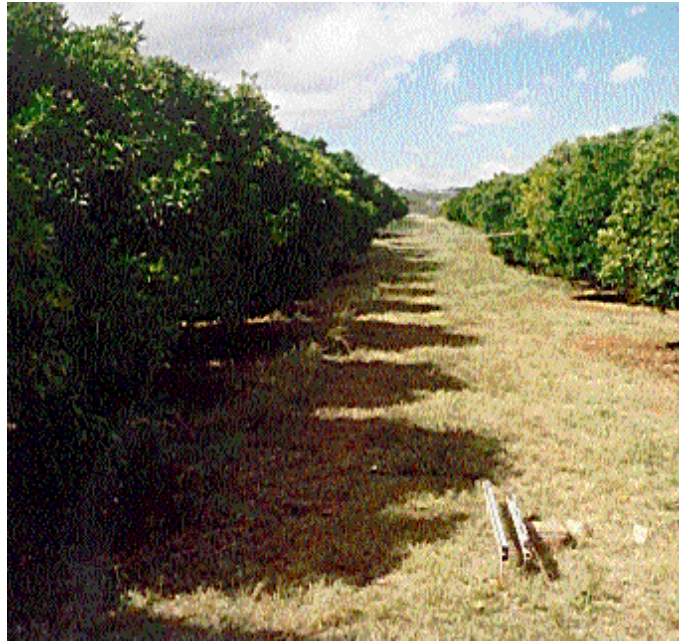
Figure 2.14. View of Clementine hedgerow and tube solarimeter in inter-row. Note the jagged shade line.
