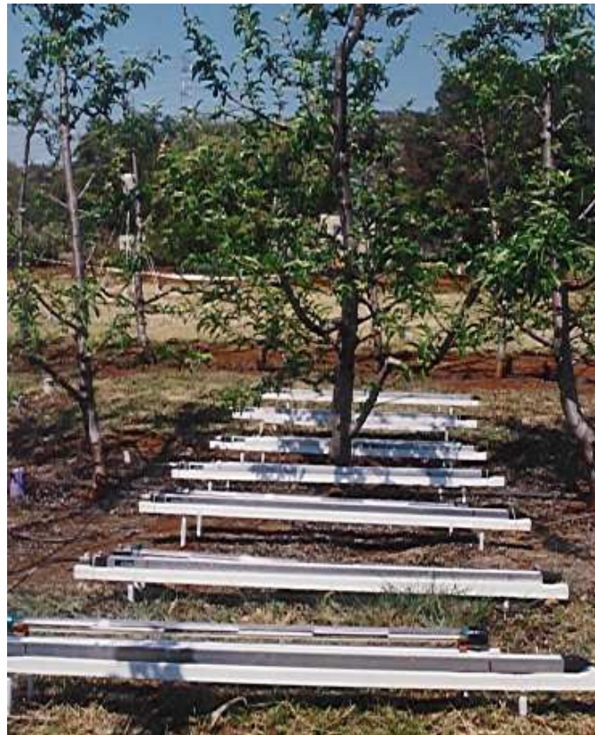
Figure 2.7. View of tube solarimeters and LQS installed under the peach hedgerow to record solar irradiance under a developing canopy.
