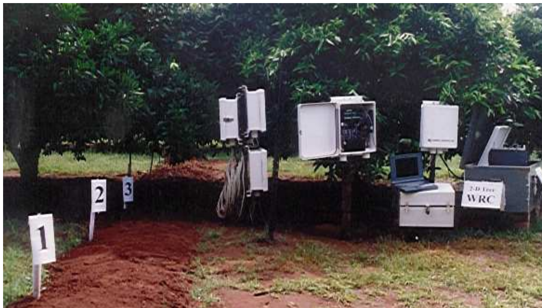
Figure 2.12. Completed installation of HDS and TDR sensors and control units in the clementine hedgerow at Syferkuil.
