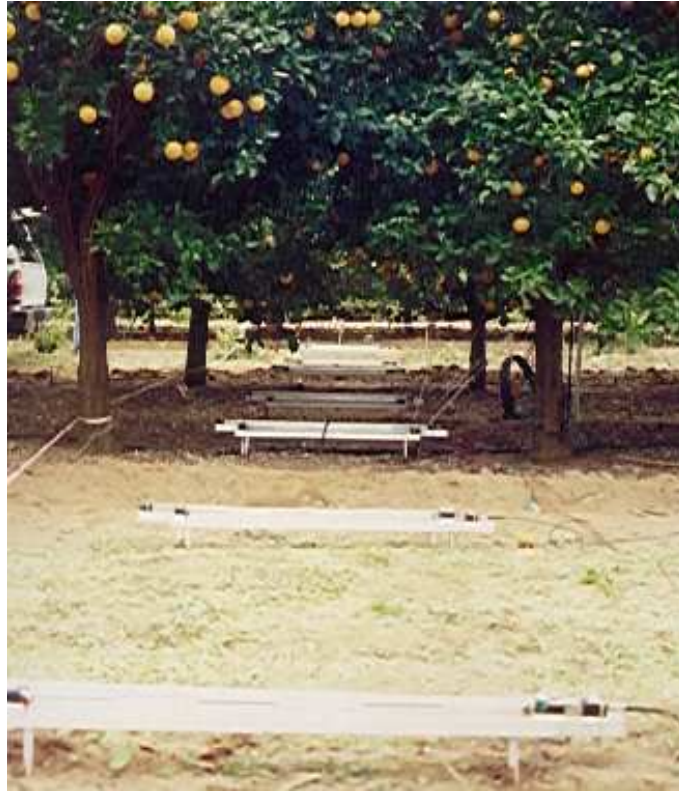
Figure 2.18. View of valencia tramline hedgerow and tube solarimeters installed under canopy to record solar irradiance under tramline canopy.
