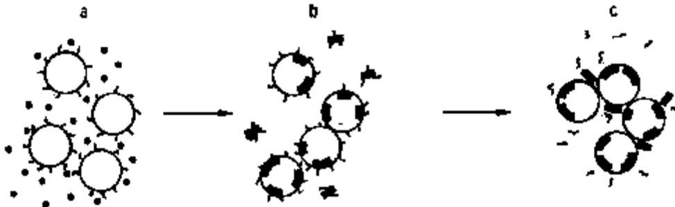
Figure 2.8: Schematic depiction of changes taking place after heating and renneting of (a) the casein micelles with CMP protrusions and native whey protein in unheated milk; (b) after heating; denatured whey protein complexed with casein micelles and dissociated casein; (c) after renneting of heated milk (van Hooydonk, 1987)
