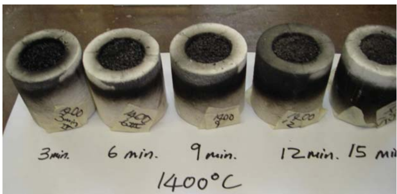
Fig. 40: No carbon deposition on crucible walls for char-ore samples
