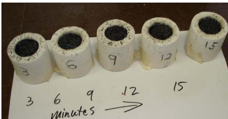
Fig. 40: No carbon deposition on crucible walls for char-ore samples
