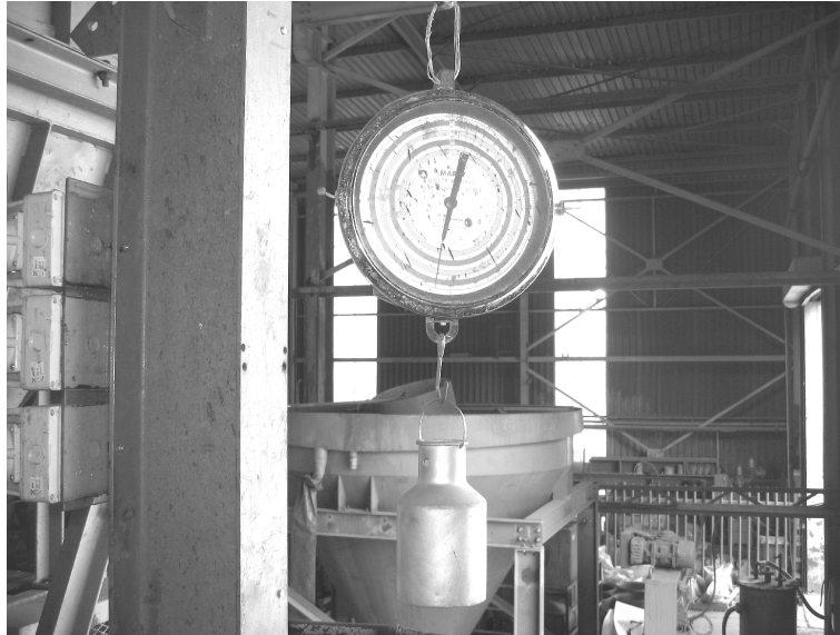
Figure A.6. The Marcy scale and 'density bottle' used to measure the medium density.
