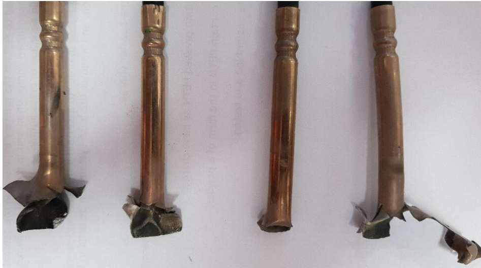
Figure 4-28. Copper-nickel shells post burn.
