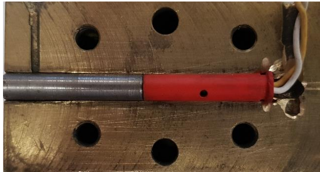
Figure 3-4. The open element housing containing an element and fuse head.
