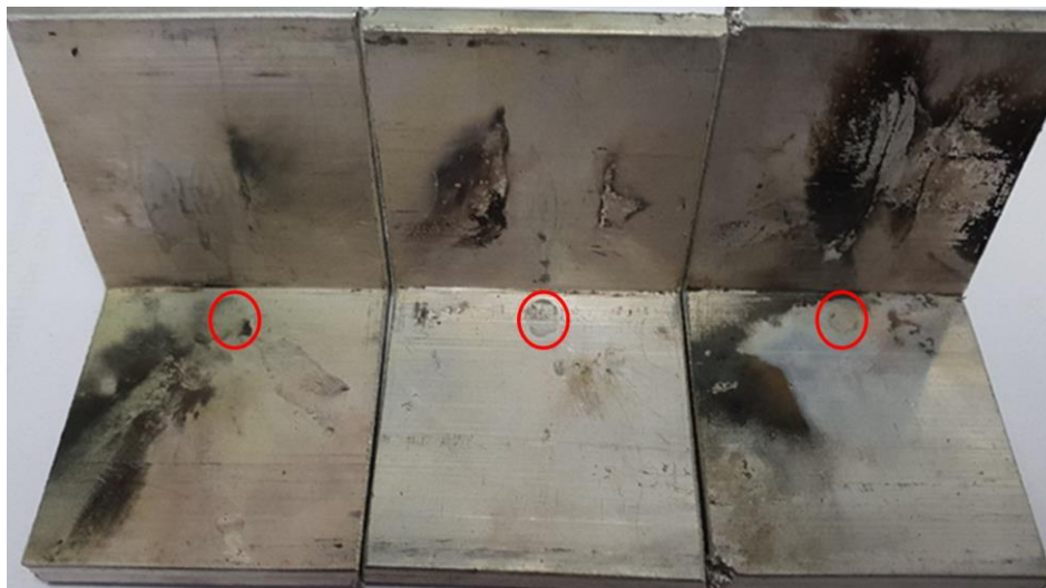
Figure 4-29. Witness plate results from detonator trials. (Dents are circled)
