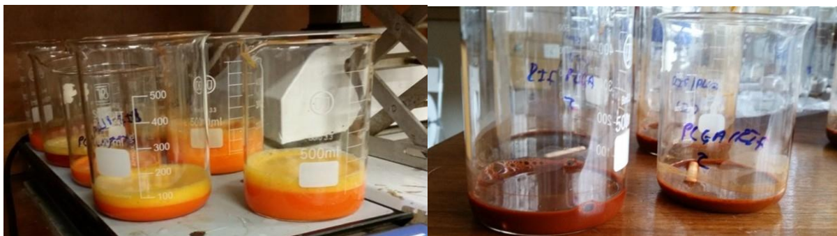
Figure 1: Representative Images of Nanoparticle Emulsions. This figure showcases representative images of the nanoparticle emulsions produced during the formulation process. The left image displays the emulsion after homogenization, while the right image shows the emulsion after overnight stirring to evaporate the solvent. These images provide a visual representation of the nanoparticles in their emulsified state.
