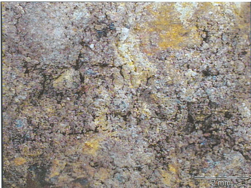
Photograph A10. 1.8% net bitumen, 2% cement, 7x magnification
