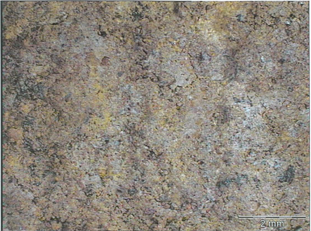
Photograph A7. 1.8% net bitumen, 1% cement, 7x magnification
