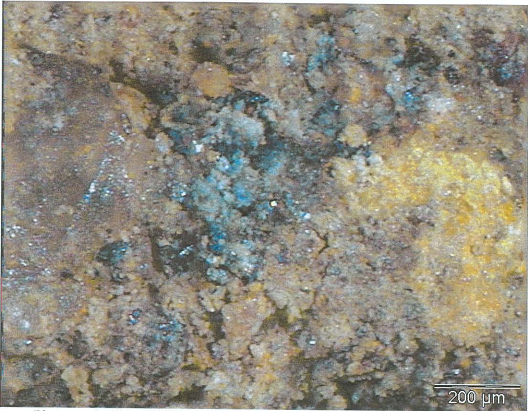
Photograph A21. HVS site sample. Bitumen with cement, 50x magnification
