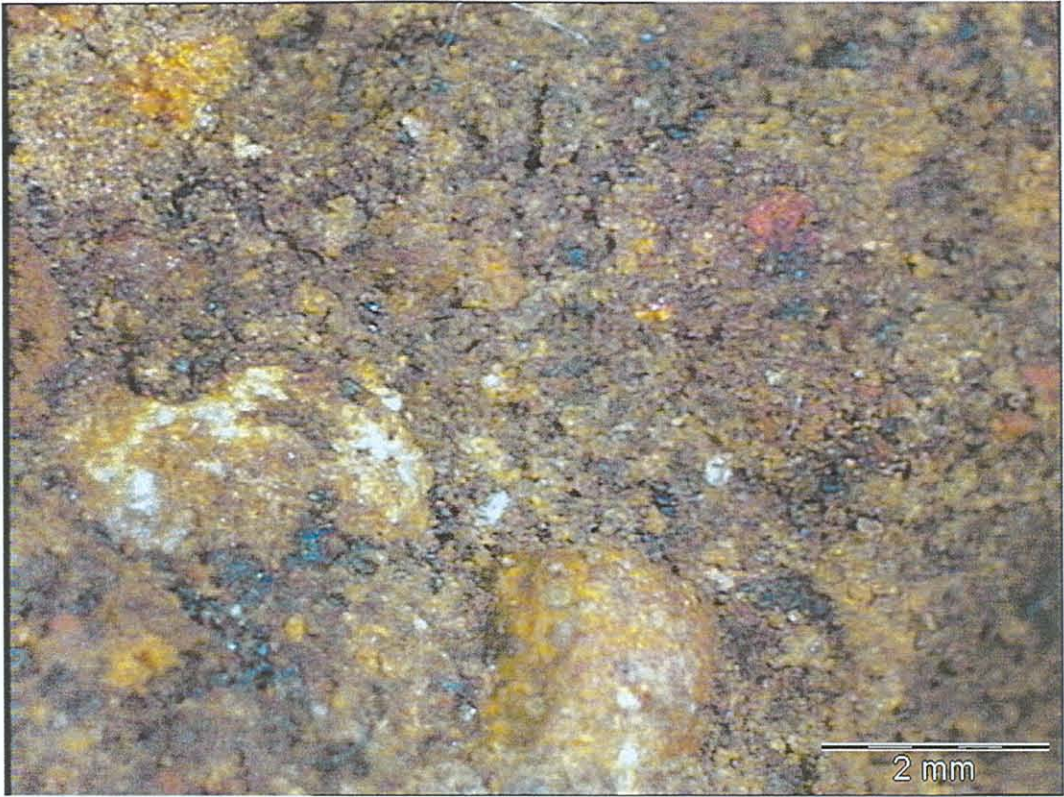
Photograph A15. 3.0% net bitumen, 1% cement, 7x magnification
