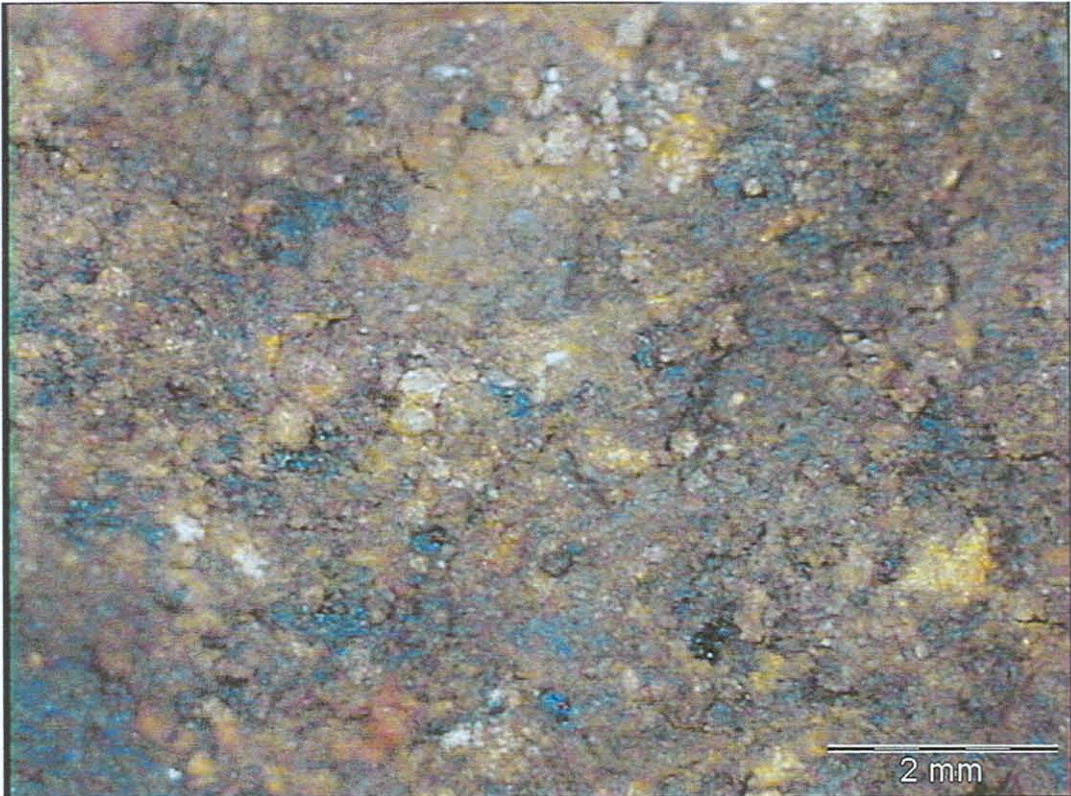
Photograph A13. 3.0% net bitumen, 0% cement, 7x magnification
