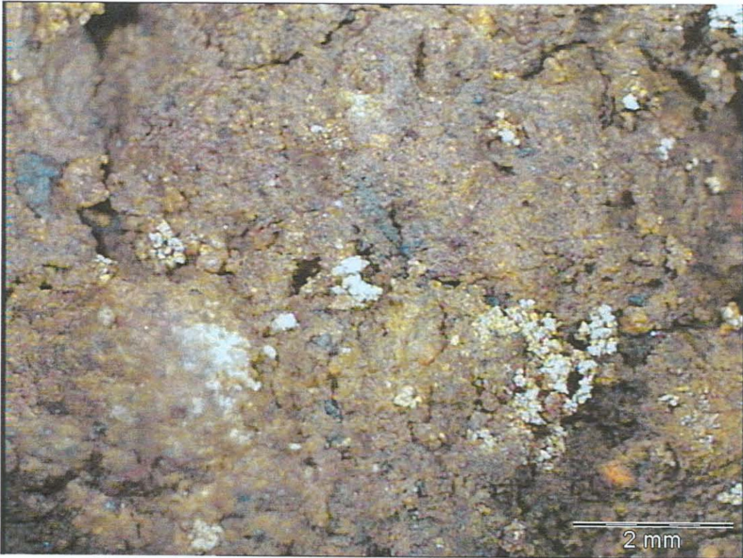
Photograph A1. 0.6 % net bitumen, 0% cement, 7x magnification
