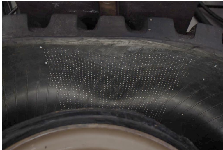
Figure 6-9 Marker position on tyre carcass (50mm cleat)
