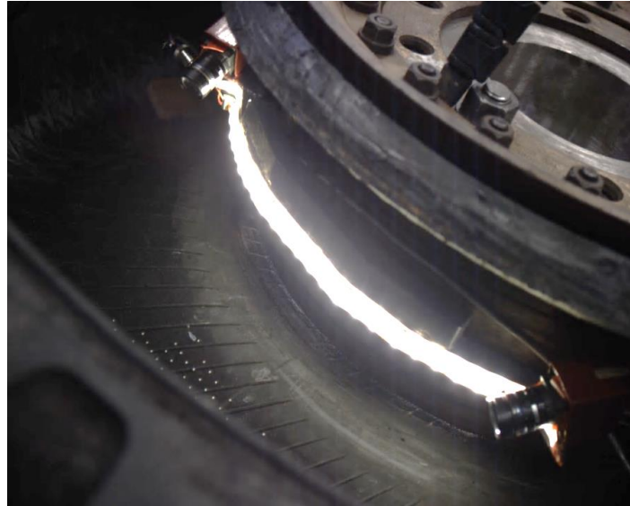
Figure 6-8 Camera test setup mounted on the inside of the tyre
