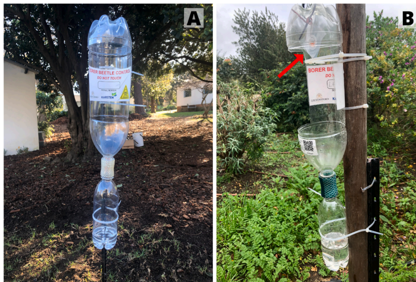
Fig. 2. (A) Front view and (B) side view of baited traps showing slow-release lure containing Quercivorol ((1S,4R)-p-menth-2-en-1-ol) (arrow).
