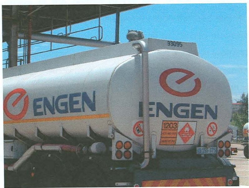
Figure 3.5 Modified road tanker to allow for vapour recovery.
