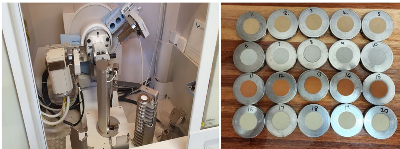
Fig. 22 PANalytical X'Pert Pro powder diffractometer (left) and XRD pressed powder samples (right) (© Jason Tunnell)
