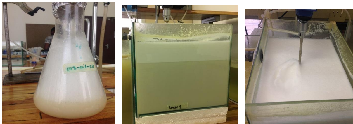
Figure 4-4: Foaming results (left=batch, center = CSTR side view, right = CSTR top view)
