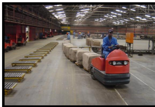
Figure 7 Electric carts used to haul trailers
