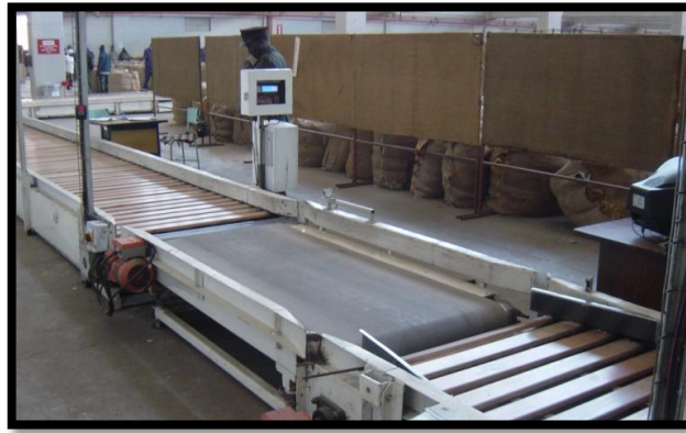
Figure 50 Scale built into Slatted Conveyor
