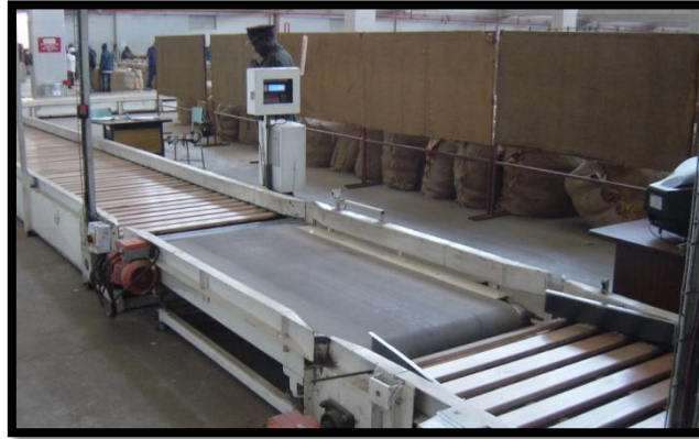
Figure 18 Built in Scale - Belt Conveyor
