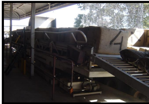
Figure 51 Scissor lift/Slatted conveyor combination
