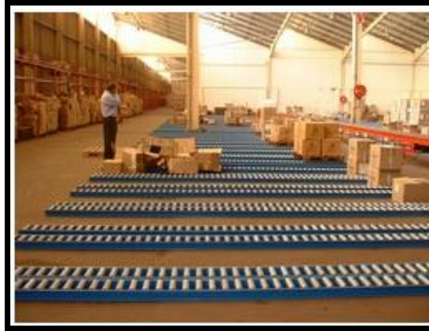
Figure 16 Ground level Roller Conveyor
