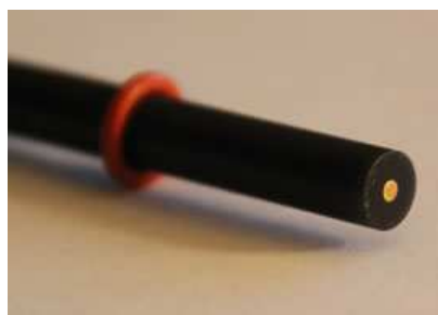
Figure 4.3: A working electrode with a gold sensor surface.
