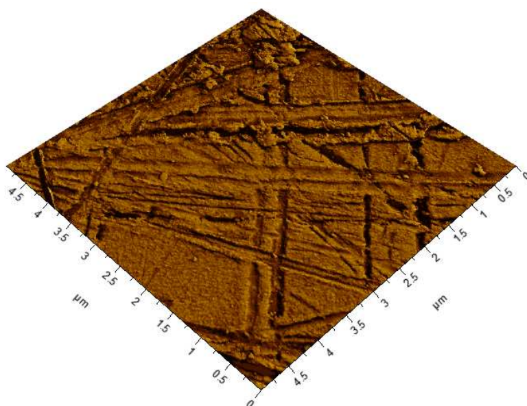
Figure 4.14: AFM phase image of SAM of MASH.
