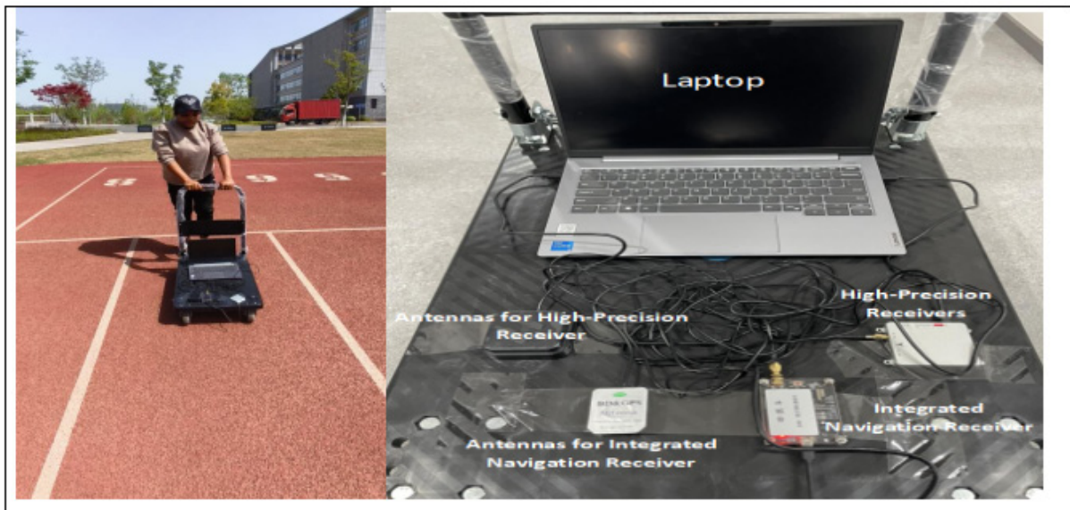
Figure 1: The author simulates a train’s motion, and the Septentrio-Mosaic receiver and Matlab for real-time data processing mirror RTK-based systems
