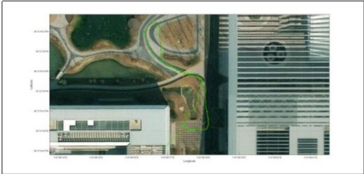
Figure 4: Trajectory comparison of Integrated GNSS/INS with RTK vs. GNSS-Only System at Beihang University Stadium (Construct, 2025)
