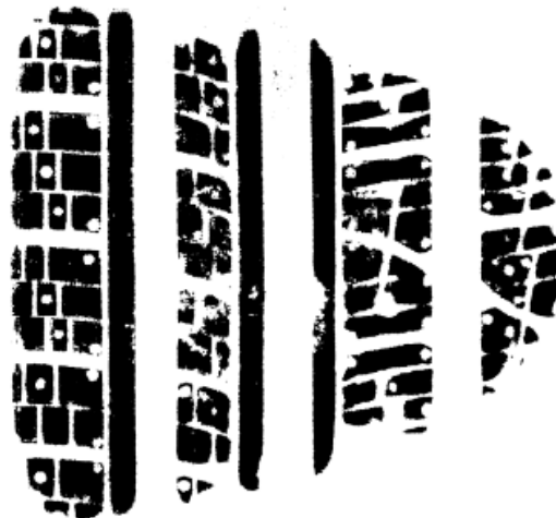
Figure 1 – Footprint on a flat surface of Pirelli Scorpion Verde 235/55 R19 105V tyre at -4° camber at 250kPa inflation pressure (Wright, 2017)
