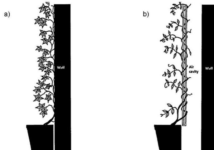
Figure 12: Green facade classification: a) Direct green facades, b) Double-skin green facades (Sheweka & Mohamed, 2012).
