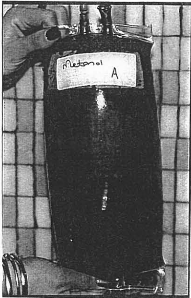
Figure 4. The anaerobic bioreactor (the expansion of the bag indicates gas production).
