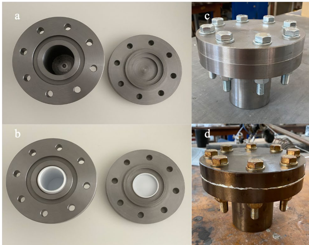
Figure 4.4: Visualisation of a) alloy steel vessel; b) vessel with the PTFE lining; c) top view of the assembled reactor; d) view of the reactor after running the first HTC test.
