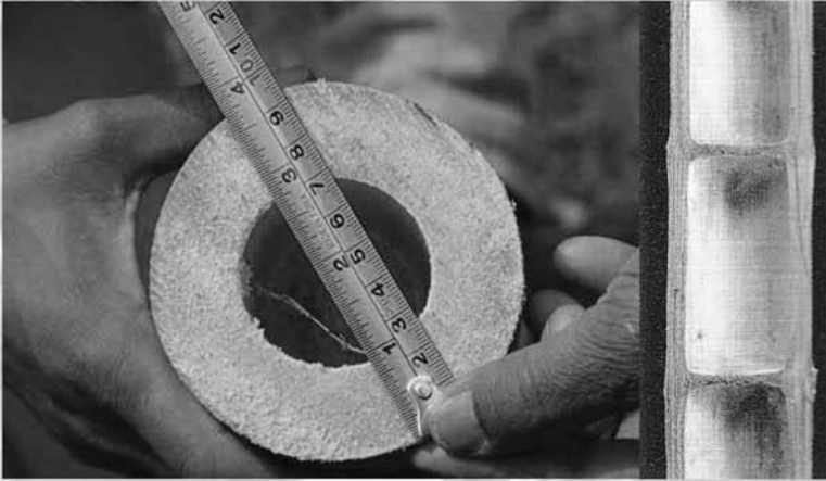
Figure 13.65 Above: Diameter of Bambusa Balcooa (NMBA 2009); section through a bamboo culm (Von Vegesack and Kries 2000:205)
