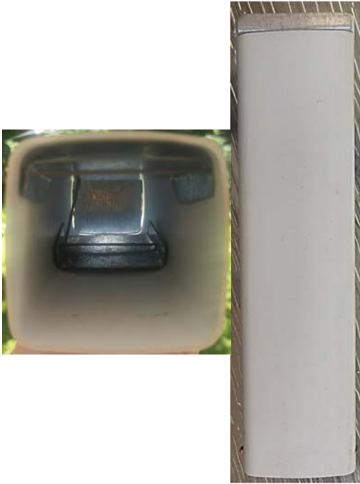
Supplementary Figure 2: Pictures of the PVC live traps used to capture small mammals. Left – front view of the trap, showing the door at the top of the trap that is kept open by a little steel arm on the lefthand side and the metal plate at the bottom of the trap that triggers the door. Right – top view of a trap.
