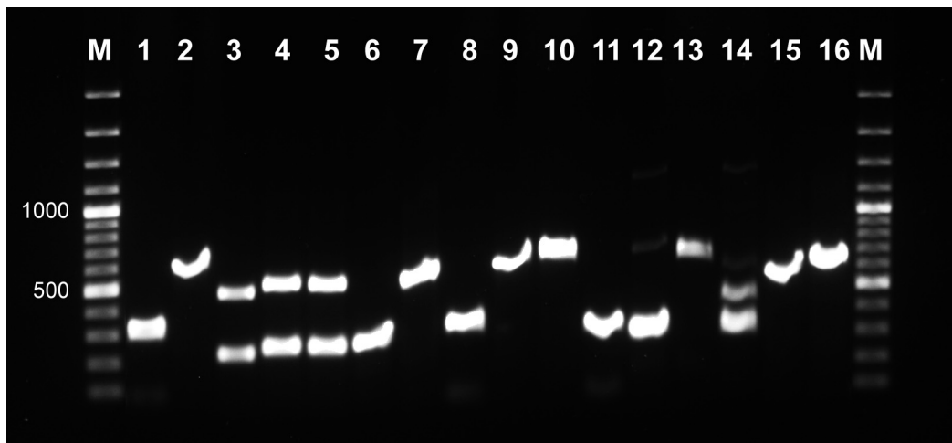
Fig. 2. Simultaneous agarose electrophoresis (1.5 % w/v) of MAT1-1-3 (higher bands - around 450 bp) and MAT1-2-1 (lower bands, about 230 pb) PCR fragments from representative Leptographium sensu lato species. G. alacris : CMW1136 (1), CMW202 (2); G. europhioides CMW446 (3); G. aenigmatica CMW2199 (4); G. piceiperda CMW2811 (5); G. koreana : CMW14200 (6), CMW14201 (7); G. huntii : CMW1006 (8), CMW1015 (9); L. bhutanense : CMW18650 (10), CMW18652 (11); L. longiclavatum : CMW20606 (12), CMW20607 (13); G. wagneri CMW53 (14); L. wagneri var. pseudotsugae CMW1533 (15); L. wagneri var. wagneri CMW1828 (16). The molecular weight marker used was GeneRuler™ 100 bp Plus DNA Ladder (Fermentas).
