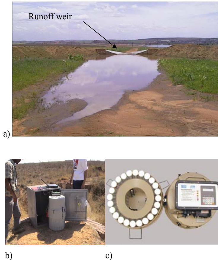
Figure 3.21 a) Runoff weir layout and b) ISCO sampler at Pivot Major and c) Top view of ISCO sampler with 24 sample bottles
