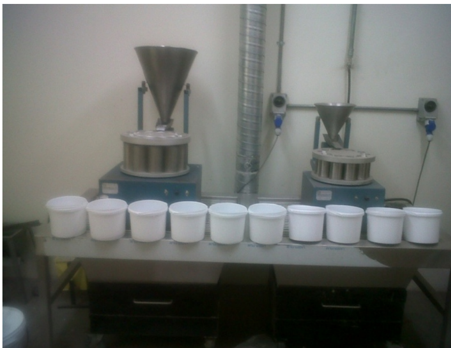
Figure 3.3: Photograph showing the rotary splitter used for the splitting of phosphogypsum into representative homogeneous sub-samples.
