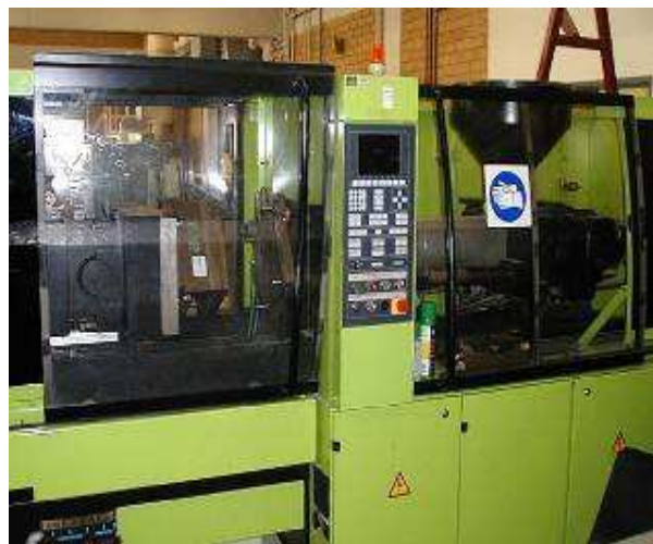
Figure 3.3: Injection moulder Engel 3040, 800 kN
