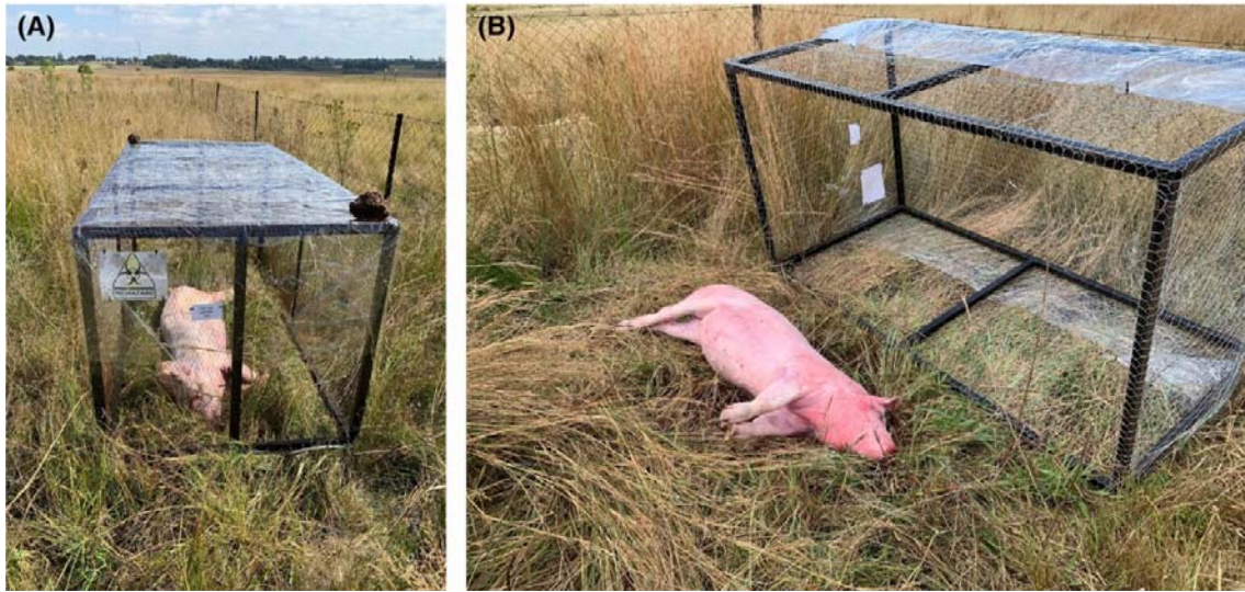
FIGURE 1. Custom metal cages, 0.9 m × 0.9 m × 2.0 m, surrounded with chicken mesh to prevent the entry of large scavengers and covered with a transparent plastic tarp, fastened to the cage, to prevent natural rehydration.
