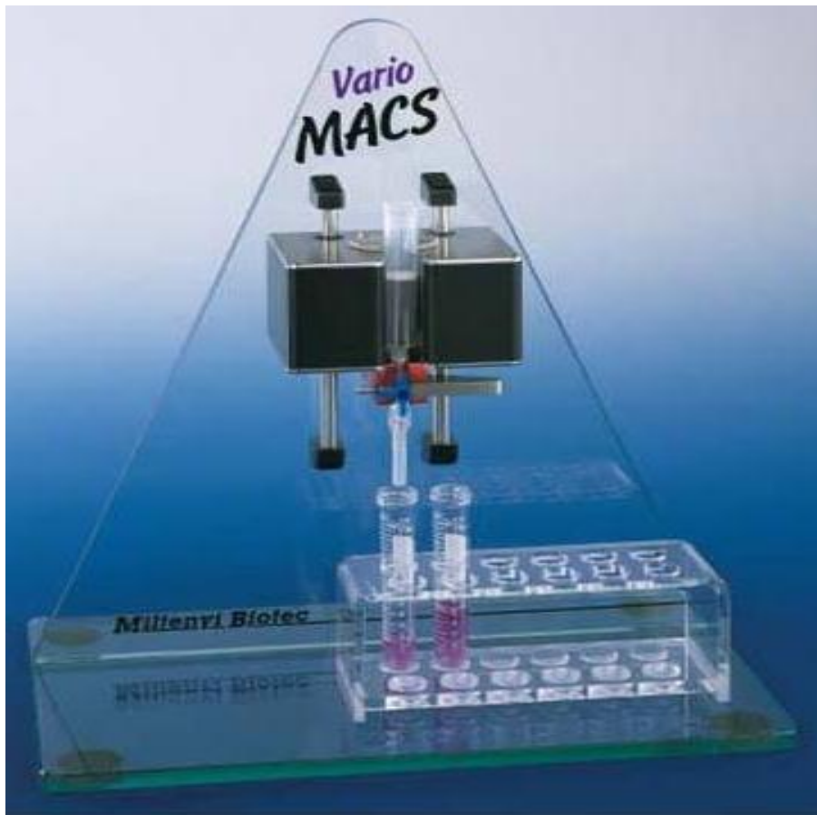
Figure 2.2: An image of the VarioMacS separating system that was used to obtain purified parasitised RBCs at the late trophozoite stage. Copyright© 2015 Miltenyi Biotec. All rights reserved (with permission).
