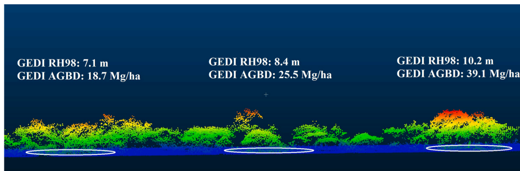
Fig. 3. Cross-section of normalized ALS point cloud data showing GEDI 25m footprints and corresponding GEDI Relative Height 98 (RH98) and GEDI L4A aboveground biomass density (AGBD).
